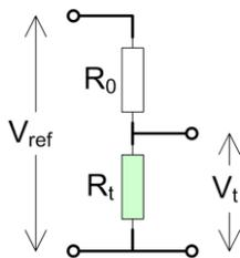
Some attention needs to be given to the desired accuracy; the ADC has 12 bits, so precision is  $V_{ref} / 4096$ . A too large value of  $R_0$  will lead to low  $V_t$  and hence coarse resolution, and with a too low value  $V_t$  will hardly change anymore. So ideally the values of  $R_t$  and  $R_0$  should be close, i.e.  $V_t$  should be targeted around half the reference voltage.
