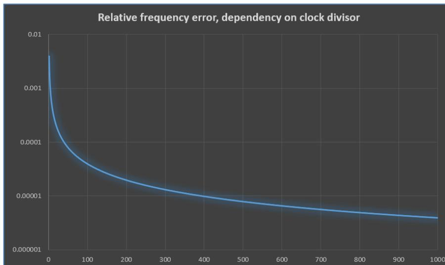
The relative error, as related to the resulting sample clock, sinks below 0.1% already at division factor 4, at factor 40 the relative error drops below 0.01% and at factor 400 even below 0.001%. The relative error of course
