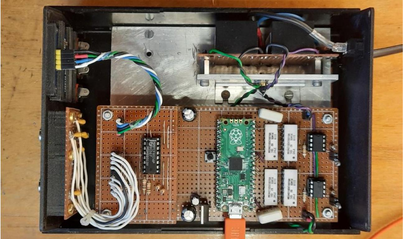
In this project, the fairly new Raspberry Pico (**RP2040**) is used to build a Signal Generator. After having gained some experience with my uSDR project, where the multi-core and signal processing were the main subject, this  $\mu$ WFG combines the very nifty Programmable I/O (PIO) feature with the flexible DMA service.
