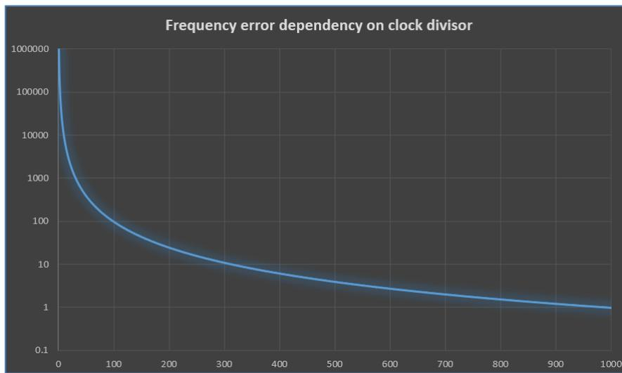
The strategy will be to maximize the number of samples in a waveform definition, where still a `sys_clk` divisor can be selected that provides reasonable precision. The maximum sample clock error is determined by the divisor step size, but it drops quite rapidly. With a `sys_clk` of 250MHz, the error drops below 100Hz when the divisor is larger than 100 and when the divisor is 300 the error is still only about 10Hz. But for small divisor values the step size can be up to 1MHz.
