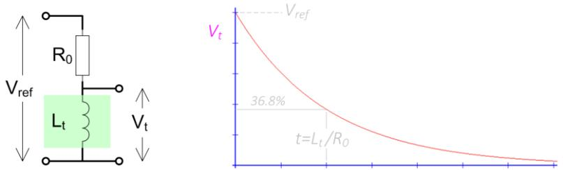
In contrast with the capacitance measurement, here the  $R_0$  value should be kept (very) low for higher accuracy. With a 1k $\Omega$  value and 200 $\mu$ sec integration time the lower limit for L is in the order of 200mH. The value of  $R_0$  cannot be lowered much more, because of the output current limitations of the Pico (max 12mA).
