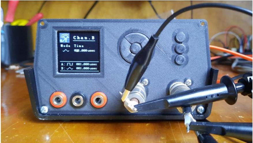
The HMI for channel settings is almost complete here for the generator part. In these images the channels A and B are set for 1usec period square and triangle waves.
