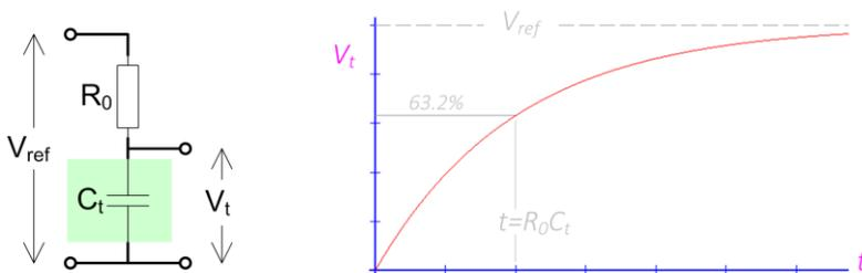
The ADC can do a measurement every  $2\mu s$ , after which the result is compared with a predefined level, more precisely the level that is reached after the RC time is over, 63%. If  $V_{ref}$  represents the full ADC range, the inaccuracy is inherently determined by the  $2\mu s$  conversion time and the  $V_{ref}/4096$  sample precision. This is best case...
