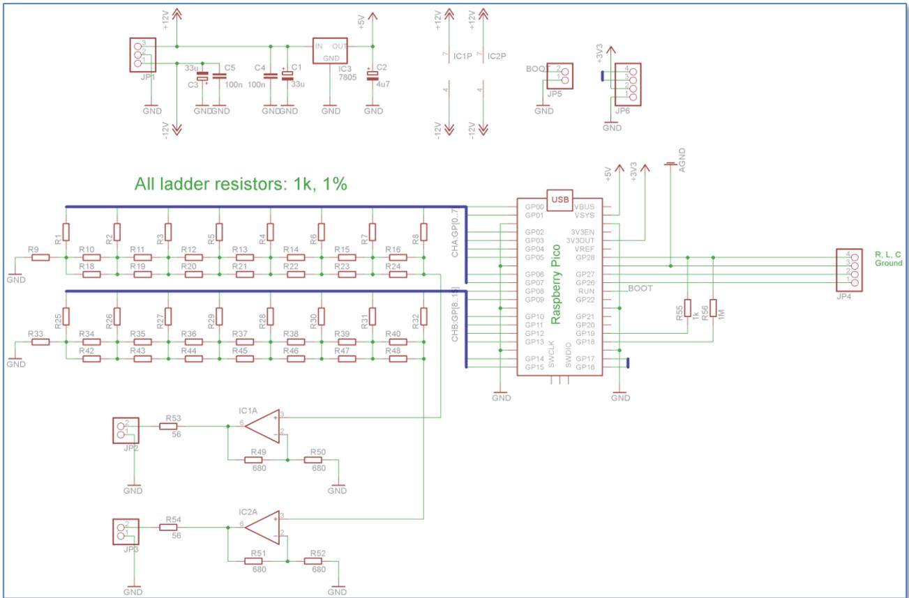
Schematic of the prototype. I have used high-speed video line drivers AD811 as analogue signal buffers. These OpAmps go up to 140MHz, and give a very good representation of the waveforms for the frequencies used.
