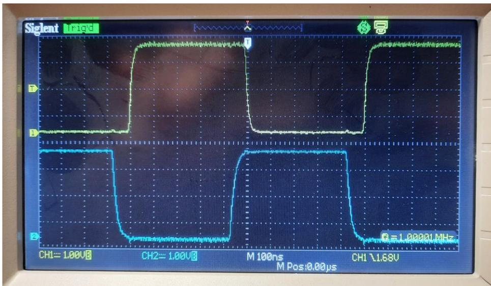
Reducing the ladder resistor in channel A to  $0.5k\Omega$  makes the edges even steeper, while the Pico can still cater for the output current.
