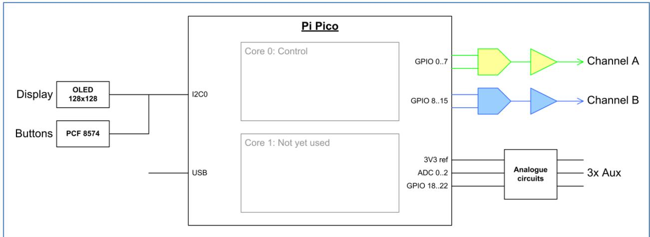
The architecture is quite simple, just the Pico and DA conversion. A serial interface is added via USB to enable file upload and control from a PC. The functionality is divided in three, a generator, a tester and a control part.
