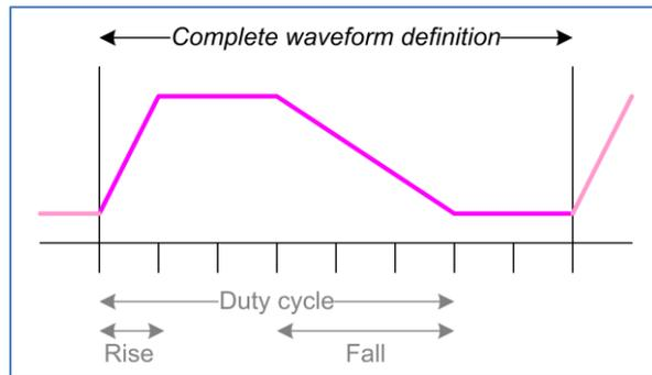
The pulse waveform is user definable, and apart from the total duration it is specified by the duty cycle, and rise/fall times. These phases are given relative to the full waveform duration, for example an upgoing sawtooth would be defined by 100% duty cycle, 100% rise time and 0% fall time.
