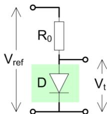
The voltage drop in forward direction ( $V_f$ ) is determined by the manufacturing technology. Schottky diodes have a  $V_f$  of lower than  $0.3V$ , Germanium diodes just over  $0.3$  and Silicon diodes closer to  $0.7V$ .
