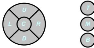
There are three auxiliary buttons (B, M, T) and four navigation buttons plus a center button (C, U, R, D, L), adding up to a full byte. Feedback to the user is given through the OLED display, which is also coupled via the I<sup>2</sup>C bus (see lcd.c).
