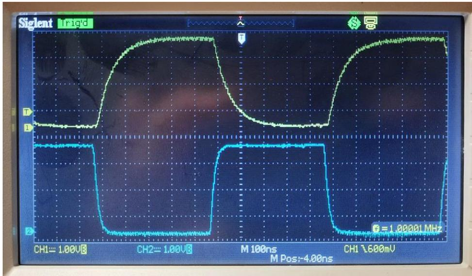
The top signal is the  $5k\Omega$  ladder, and the bottom the  $1k\Omega$  ladder. Clearly, the higher resistance network is more susceptible to parasitic capacitance, while the low resistance network can still be sufficiently driven by the Pico outputs. When the frequency is increased, the longer rise and fall times in channel A result in reduction of the signal amplitude. Possibly, this can be compensated by increasing the buffer circuit input impedance, and make this frequency dependent.
