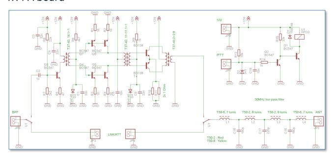
The transmitter PA board is still highly under development. The idea is to have a wideband linear driver as proposed by Harry Lytthal (SMOVPO) that outputs up to 500mW. The end-stage, also class AB push-pull configuration, should be good for a few Watts, but still needs to be tried out.
