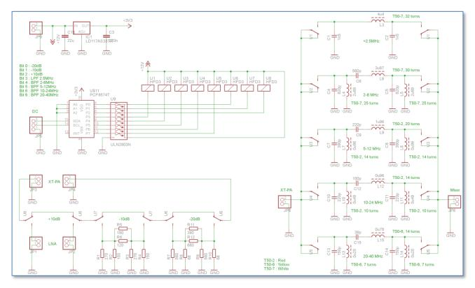
The 5 band filters and the attenuators/LNA are selected through relays, controlled from the Pico via the I<sup>2</sup>C bus.
