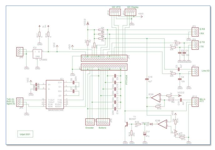
The processor board hosts the Pico module and all user I/O. There is also a serial interface that receives a monitor with a command line interface. The PTT is generated either from a hard signal from a microphone, or by a level detection circuit in case of e.g. computer generated FT-8 encoding.
