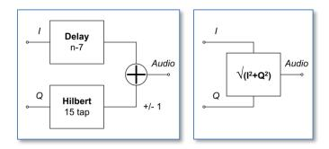
For SSB demodulation, the decimated I and Q samples are stored in a 15-sample delay line. A 15-tap Hilbert transform on the Q channel is done and the result is subtracted from or added to the n-7 sample in the I delay line to obtain the USB or LSB audio output.
