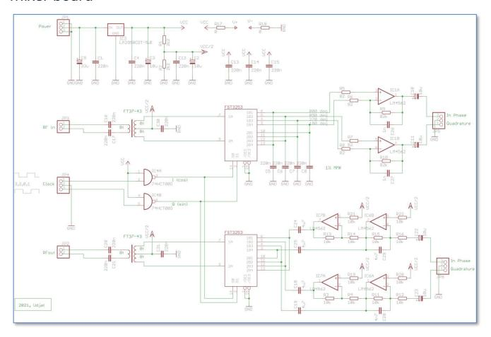
The mixer board hosts the two mixers, QSD for RX branch and a QSE for the TX branch. The switches are clocked from the Si5351 board, through two NAND gates that take care of level shifting and some signal cleanup.
