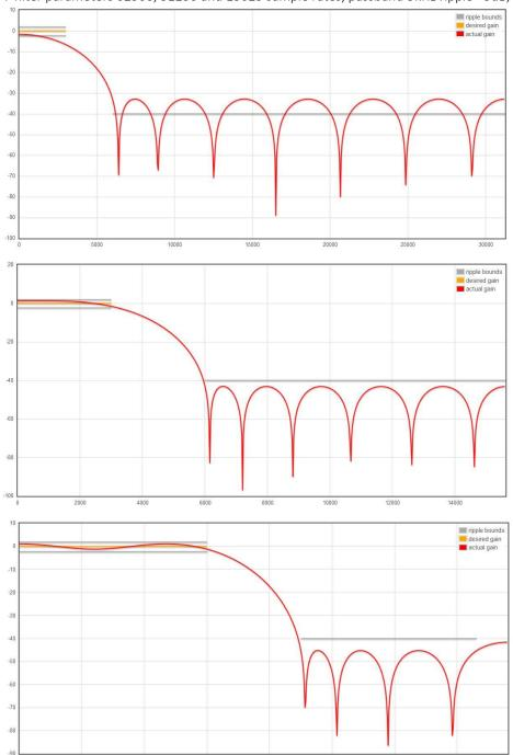
Note that for the 3kHz low pass filter, a 15 tap FIR algorithm works best at lower sample rates. For high sample rates it would be better to use more taps.
