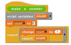
This script implements an object *class*, a type of object, namely the counter class. In this first simplified version there is only one method, so no explicit message passing is necessary. When the **make a counter** block is called, it reports a procedure, the ringed script inside its body. That procedure implements a specific counter object, an *instance* of the counter class. When invoked, a counter instance increases and reports its count variable. Each counter has its own local count:
