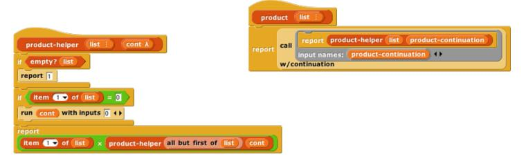
The **call continuation** block takes as its input a one-input script, as shown in the **product** example. It calls that script with *the continuation of the call-with-continuation block itself* as its input. In this case, that continuation is
