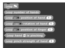
The LEAP Motion controller is a piece of hardware that senses the position of the user's hands, modeling the angles of each knuckle. It's one of many external devices that Snap! can support. Generally, to use a device with Snap!, you must download and install a separate controller program. That's true for the LEAP too, but that controller is installed as part of setting up the device, so all that's needed is the block library to go with it.
