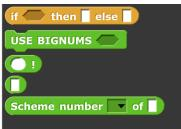
The **USE BIGNUMS** block takes a Boolean input, to turn the infinite precision feature on or off. When on, all of the arithmetic operators are redefined to accept and report integers of any number of digits (limited only by the memory of your computer) and, in fact, the entire Scheme numeric tower, with exact rationals and with complex numbers. The **Scheme number** block has a list of functions applicable to Scheme numbers, including subtype predicates such as
