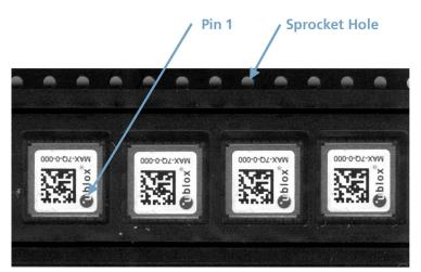
Figure 4: Tape and module orientation
