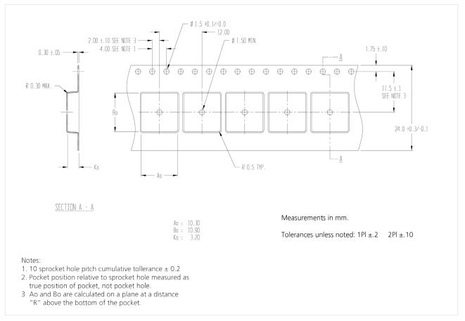
Figure 5: MAX-7 Tape dimensions
