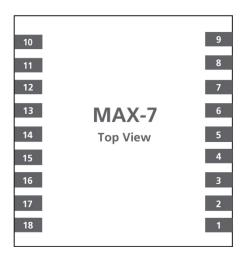
Figure 2: Pin Assignment
