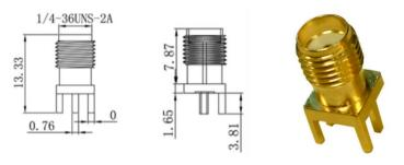
Figure 8 CaribouLite SMA connectors
