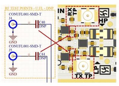
Figure 10 RF test-points
