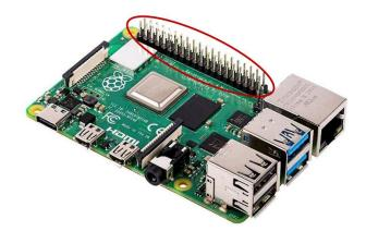
Figure 3 Raspberry Pi pins
