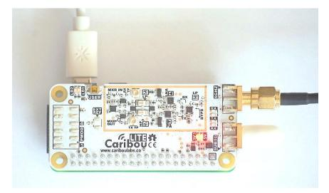
Figure 4 Powered-on CaribouLite + RPI Zero
