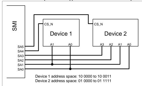
Or if fewer devices are fitted it is possible to support devices with more address pins.
