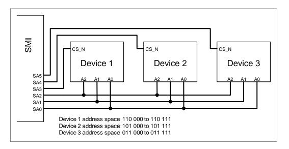
Figure 2 Three Devices With Three Address Pins
