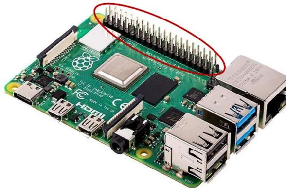
*Figure 3 Raspberry Pi pins*
