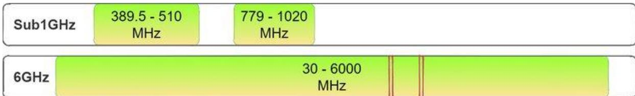
Figure 2 CaribouLite Operational frequency ranges (Tx & Rx)
