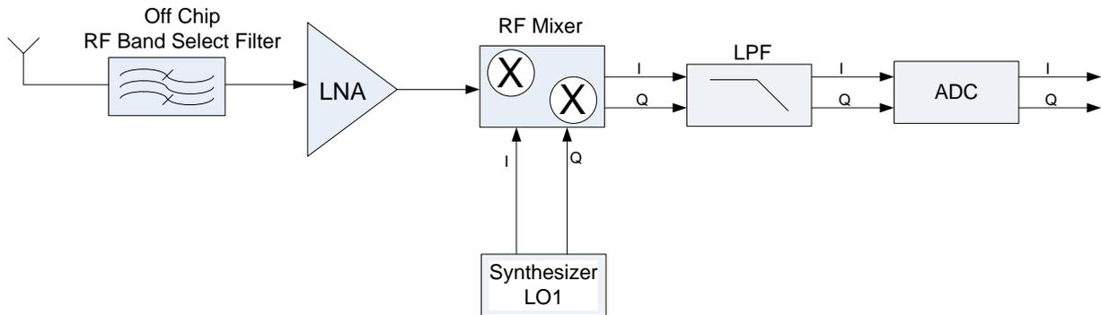
Fig. 5: Direct Conversion Receiver Architecture
