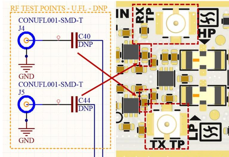
Figure 10 RF test-points
