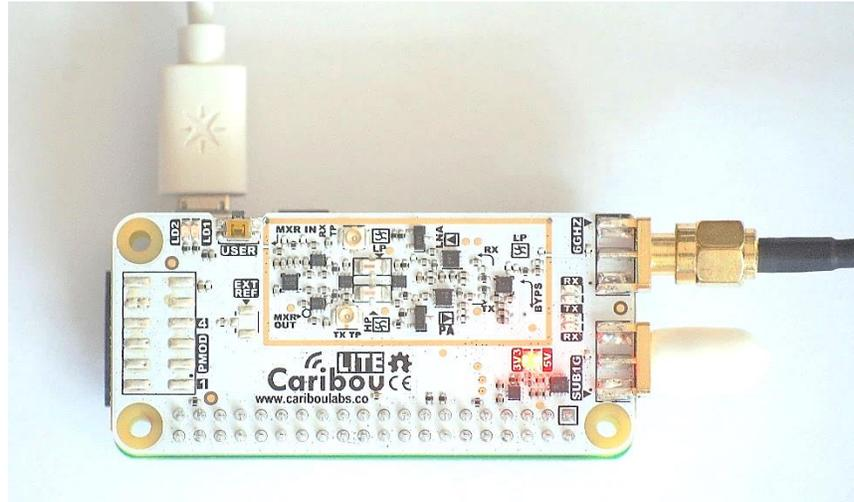
Figure 4 Powered-on CaribouLite + RPI Zero
