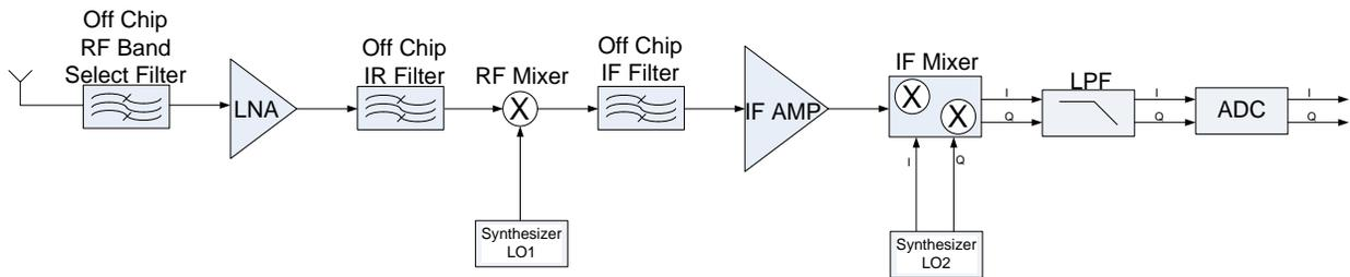
**Fig. 4: Superheterodyne Receiver Architecture**
