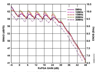
Figure 12. SINAD/ENOB vs. RxPGA Gain and Frequency
