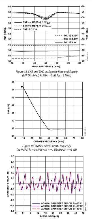
Figure 20. RxPGA Gain Step Error vs. Gain ( $f_{IN} = 10 \text{ MHz}$ )
