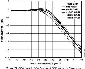
Figure 72. Effects of RxPGA Gain on LPF Frequency Response ( $f_{-3 dB} = 32 MHz$  (@ 0 dB and  $f_{ADC} = 80 MSPS$ )
