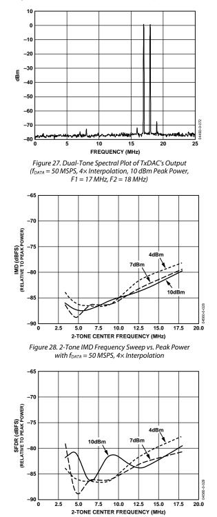
Figure 29. 2-Tone Worst Spur Frequency Sweep vs. Peak Power with  $f_{DATA} = 50$  MSPS, 4× Interpolation
