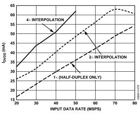
Figure 79. Digital Supply Current Consumption vs. Input Data Rate  $(DVDD = DRVDD = 3.3 V \text{ and } f_{OUT} = f_{DATA}/10)$
