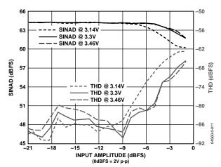
Figure 11. SINAD and THD vs. Input Amplitude and Supply  $(f_{IN} = 8 \text{ MHz}, \text{LPF } f_{-3 dB} = 26 \text{ MHz}; \text{RxPGA} = 0 \text{ dB})$
