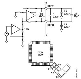
Figure 75. ADC Reference and Decoupling
