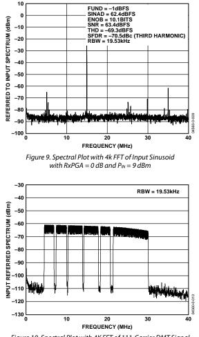
Figure 10. Spectral Plot with 4K FFT of 111-Carrier DMT Signal with PAR = 11 dB,  $P_{IN} = -33.7$  dBm, LPF's  $f_{-3dB} = 32$  MHz and RxPGA = 36 dB
