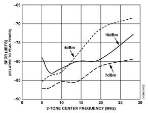
Figure 32. 2-Tone Worst Spur Frequency Sweep vs. Peak Power with f<sub>DATA</sub> = 80 MSPS, 2× Interpolation
