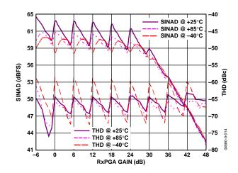
Figure 14. SINAD/THD Performance vs. RxPGA Gain and Temperature ( $f_{\rm IN} = 10$  MHz)
