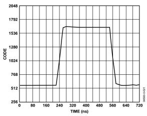
Figure 21. RxPGA Settling Time – 12 dB to +48 dB Transition for DC Input  $(f_{ADC} = 50 \text{ MSPS}, LPF \text{ Disabled})$
