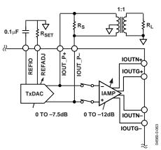
Figure 63. TxDAC Output Directly via Center-Tap Transformer
