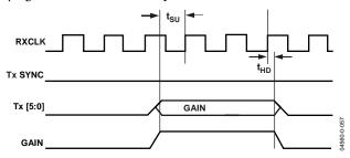
Figure 57. Updating RxPGA via Tx[5:0] in Full-Duplex Mode
