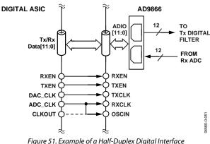
Figure 51. Example of a Half-Duplex Digital Interfo with AD9866 Serving as the Slave
