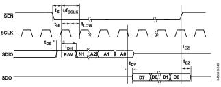
Figure 48. SPI 4-Wire Read Operation Timing
