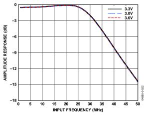
Figure 22. Rx Low-Pass Filter Amplitude Response vs. Supply  $(f_{ADC} = 50 \text{ MSPS}, f_{-3 dB} = 33 \text{ MHz}, RxPGA = 0 dB)$
