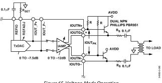
Figure 65. Voltage-Mode Operation
