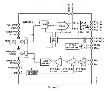
or to an internal low distortion current amplifier. The current amplifier (IAMP) can be configured as a current- or voltagemode line driver (with two external npn transistors) capable of delivering in excess of 23 dBm peak signal power. Tx power can be digitally controlled over a 19.5 dB range in 0.5 dB steps.
