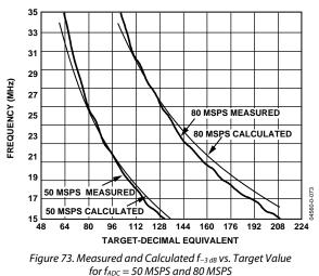
$^1$  Empirically derived for a  $f_{^{-3\,dB}}$  range of 15 MHz to 35 MHz and  $f_{\text{ADC}}$  of 40 MSPS to 80 MSPS with an RxPGA = 0 dB.
