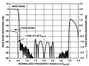
Figure 61. Frequency Response of 4× Interpolation Filter (Normalized to f<sub>DATA</sub>)
