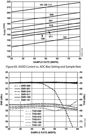
Figure 84. SNR and THD Performance vs.  $f_{ADC}$  and ADC Bias Setting with RxPGA = 0 dB,  $f_{IN} = 10$  MHz, AIN = -1 dBFS
