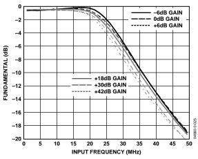
Figure 25. Rx Low-Pass Filter Amplitude Response vs. RxPGA Gain  $(LPF's f_{-3 dB} = 33 MHz)$
