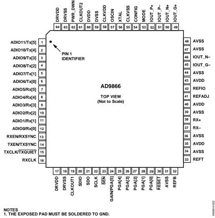
Figure 2. Pin Configuration
