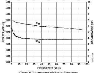
Figure 26. Rx Input Impedance vs. Frequency
