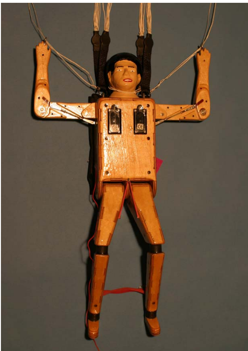
ANDY is a bit taller than MIKE. The wooden legs are quite heavy, but that helps to get the centre of gravity in the right place.
