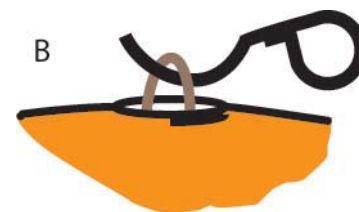
Loop A is the loop that keeps the container closed during freefall. Loop B is there for safety reasons. When you close the container, close it step by step according to numbers 1 to 4. Don't forget to pull loop B through the holes as you work along. Finally lock the container with a locking pin as shown in the little drawing on the left. This locking pin is tied to one end of a „static line“ whose other end is attached to the jump plane. When the jumper is released, the static line pulls the locking pin out of loop B. During free fall, the rc-pilot can deploy the canopy at any moment desired by releasing loop A.
