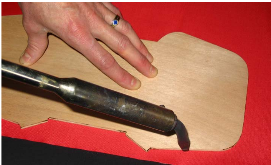
Using a soldering iron for cutting out parts for a container. The fabric is called „Parapack“, the template is made from 4 mm plywood.
