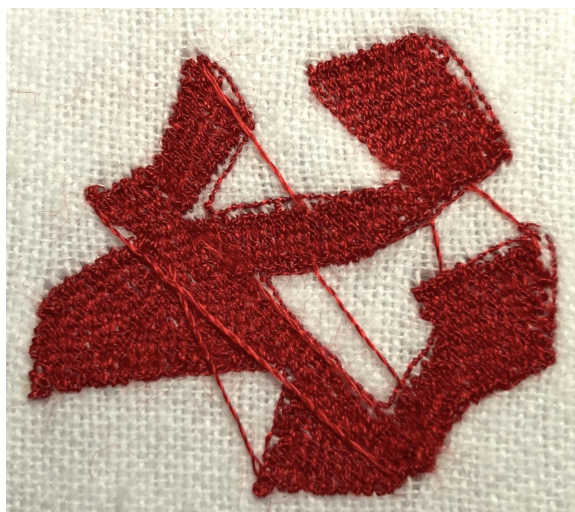
Figure 3.10: The results of stitching the finished PES file on a Brother SE600 sewing machine. The jump stitches are visible on the shape. These are necessary so the machine can reach every region on the shape and are manually cut away after the machine has finished. This is to be expected when embroidering.
