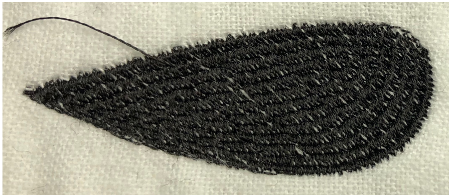
Figure 5.9: The benchmark with the max stitch distance set to 20 (2mm).
