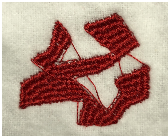
Figure 5.4: The embroidered zigzag shape. The jump stitches have not been cut away and are still visible in the photo.
