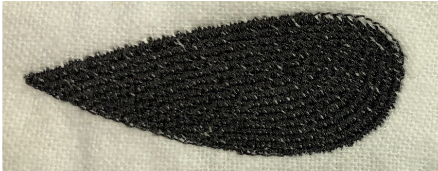
Figure 5.10: The benchmark with the max stitch distance set to 15 (1.5mm).
