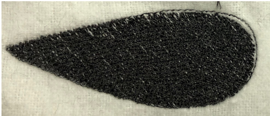
Figure 5.11: The benchmark with the max stitch distance set to 10 (1.0mm).
