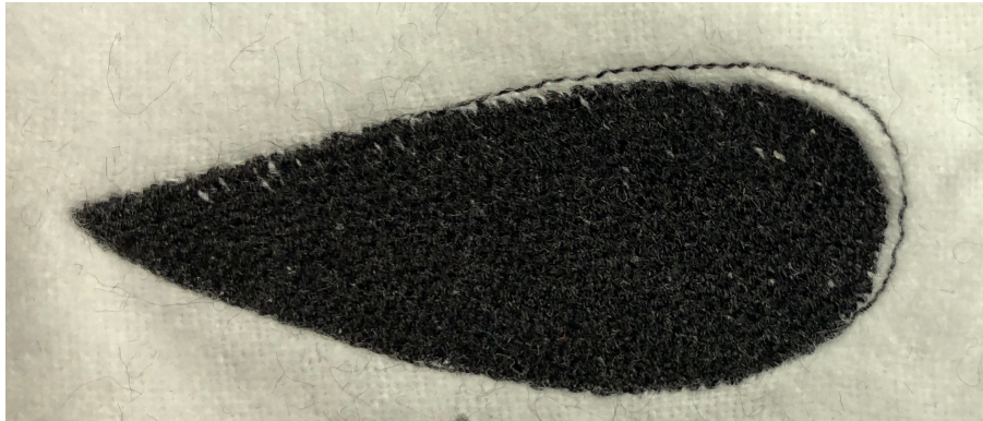
Figure 5.8: The droplet embroidered with a thread width of 1.5 (0.15mm).
