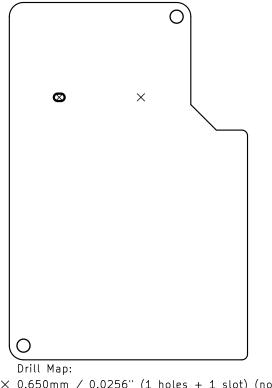
× 0.650mm / 0.0256" (1 holes + 1 slot) (not plated) O 1.152mm / 0.0454" (2 holes) (not plated)
